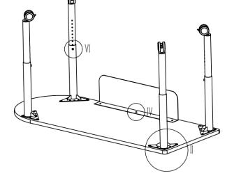
Install the front panel: 4pcs x M5x20 wood Screw
